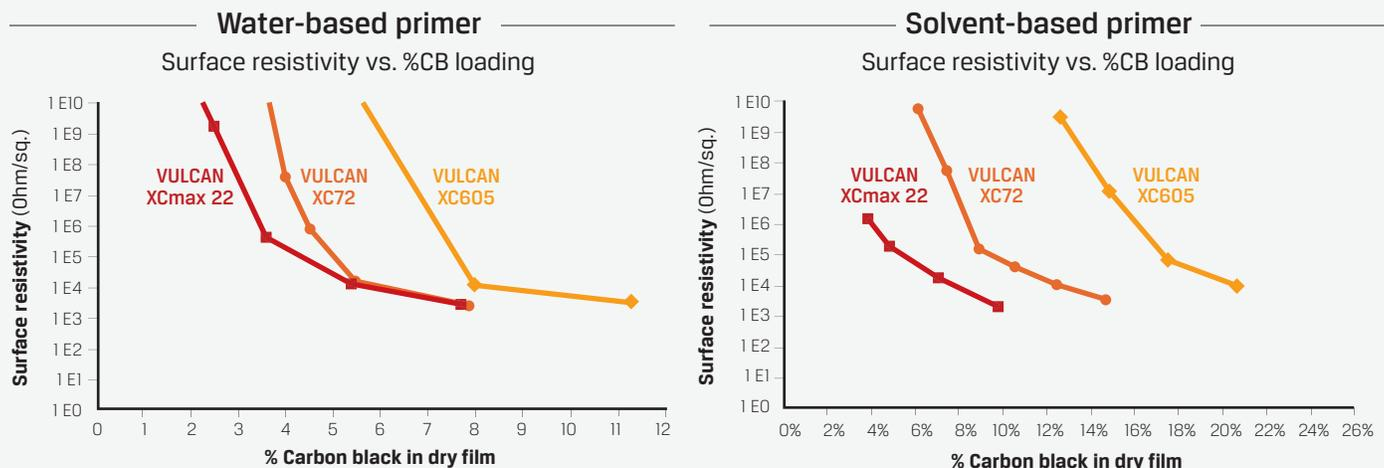
\* Surface resistivity measurement obtained using Jandel Cylindrical four point probe coupled with Keithley 2410-C source meter. Surface resistivity range of 10<sup>3</sup> – 10<sup>10</sup> Ohm/sq.
